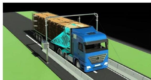
The antennas are responsible for emitting the multi-polarized electromagnetic waves generated by the microwave unit within the IMG-S Cabinet. These waves pass through the load, where they are received by antennas positioned on the opposite side, enabling accurate measurement of material properties.
