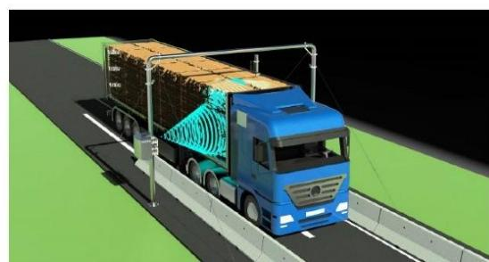
The antennas are responsible for emitting the multi-polarized electromagnetic waves generated by the microwave unit within the IMG-P Cabinet. These waves pass through the load, where they are received by antennas positioned on the opposite side, enabling accurate measurement of material properties.
